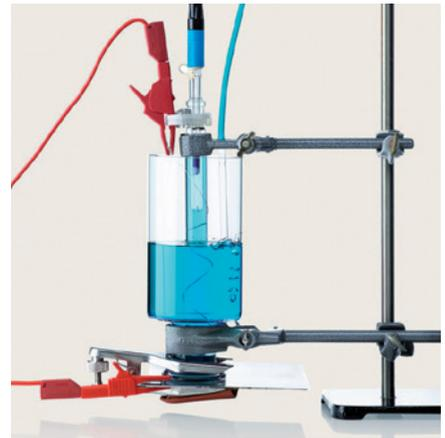
Electrochemical impedance spectroscopy equipment
